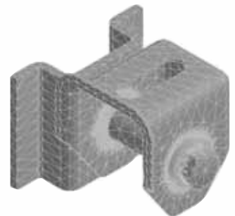
Advanced meshing with automatic contact mesh sizing offers robust meshing solutions for bracket assembly.
